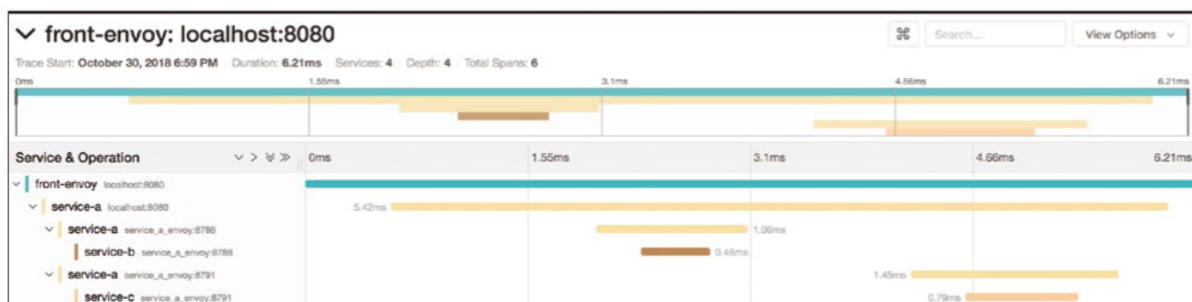
Figure 6: The Istio Envoy component links up well with Jaeger to represent and track traffic flows visually. © Arvind Thangamani
